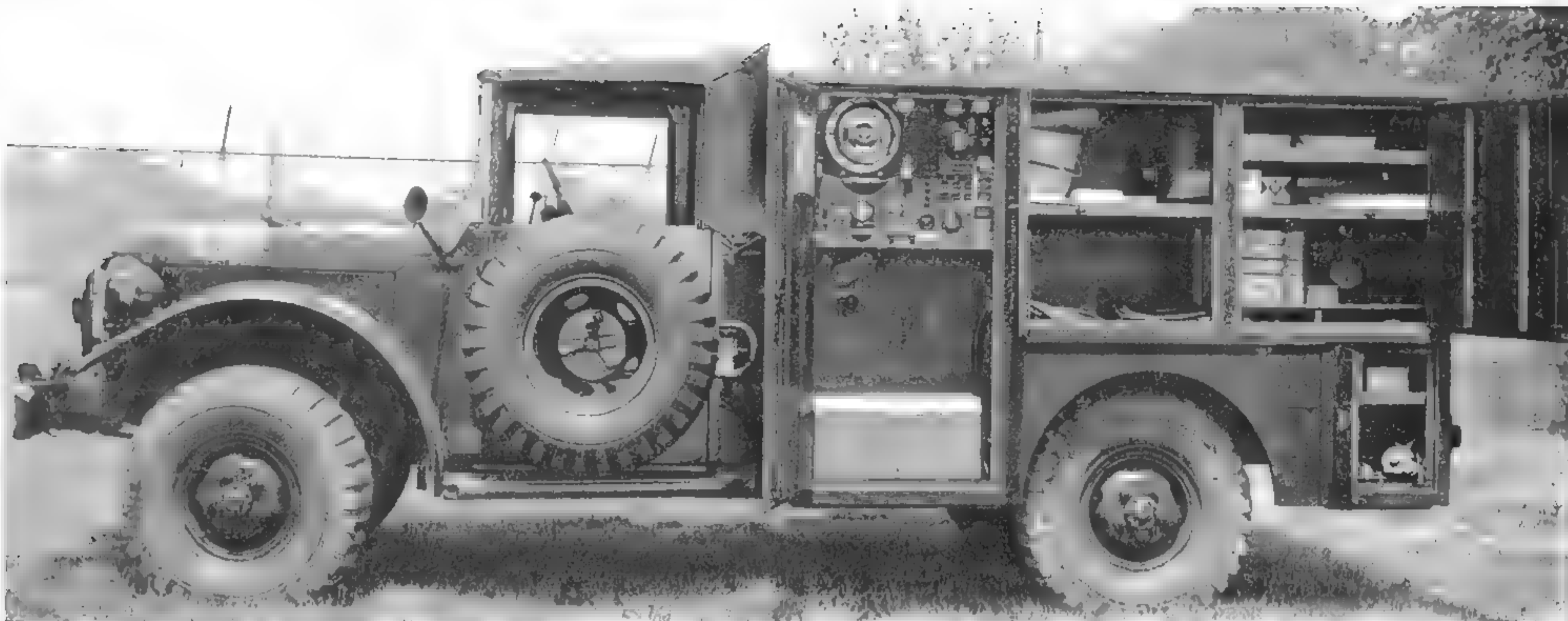
The later CMU-5 featured an aluminum body, as well as the door-type spare tire carrier characteristic of the B1 series vehicles. As can be seen in this photo, contact maintenance trucks carried an extensive, and heavy, array of tools. Notice the CMU-5 lacks the spotlights of the CMU-3. (Photo courtesy of Keco Industries)
